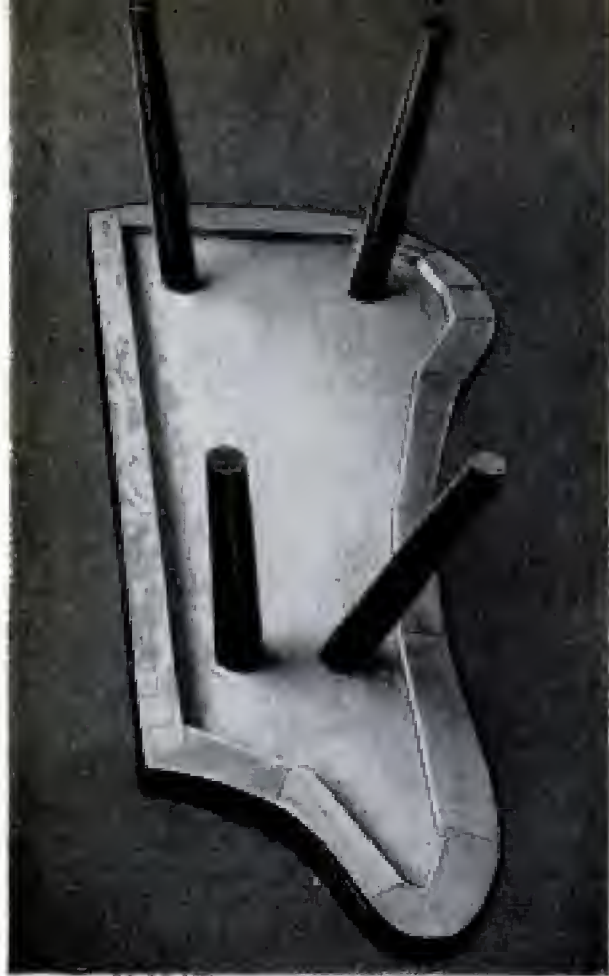
Above, underside view of table, showing how edges are built up from scraps. Below, after cork is applied to edges, it is held in place with masking tape
